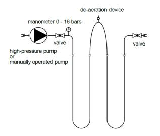
Figure 3: Basic pressure test procedure. Test procedure in detail (Fig.4 overleaf):
