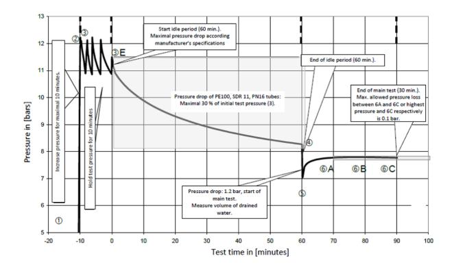
Figure 4: Detailed pressure test procedure
