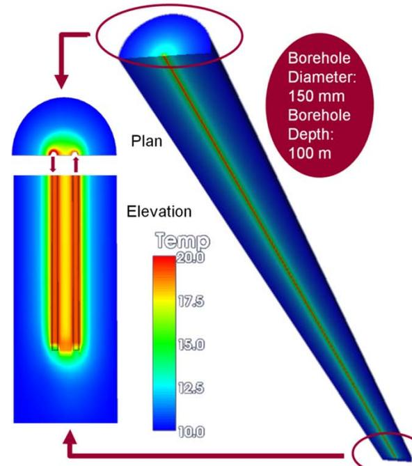
Fig. 3 Visualization of a borehole heat exchanger.
