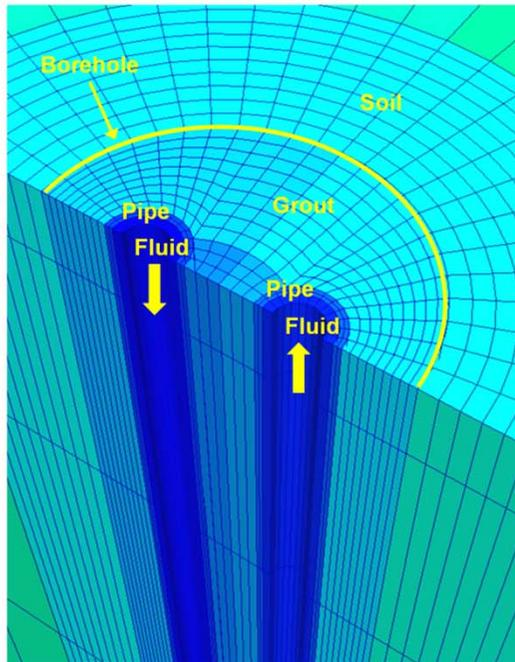
Fig. 2 Multi-block boundary fitted mesh.
